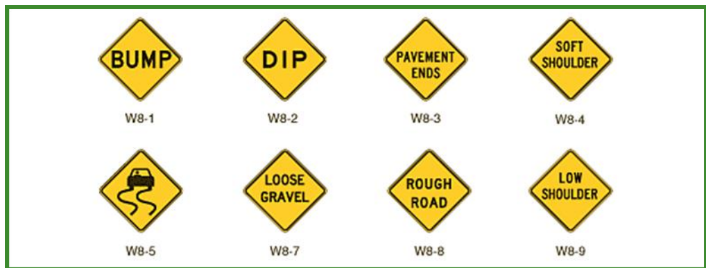
▲ A sample of some of the roadway condition signs that are especially pertinent to motorcyclists. (Source: Figure 2C-4 of the Federal MUTCD )
