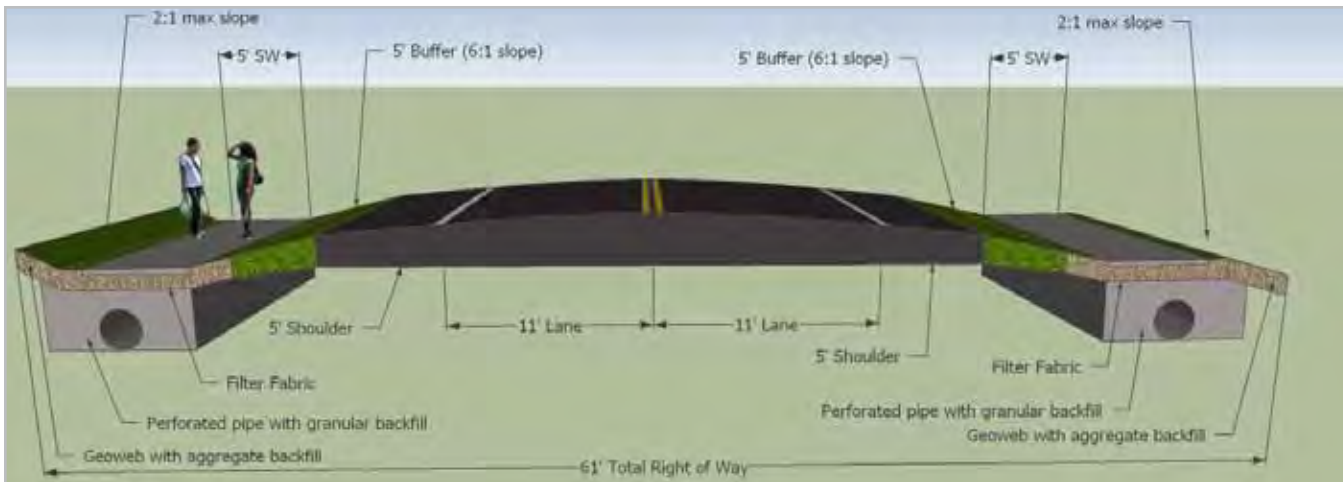
Example of road cross-section with a reduced drainage solution. Source: MORPC.
