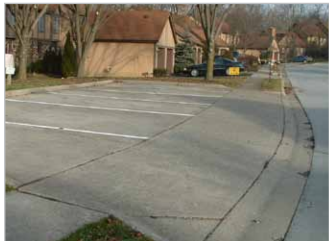
A wide parking lot entrance in front of an apartment building causes a long interruption in the sidewalk. Source: MORPC. Columbus, OH.
