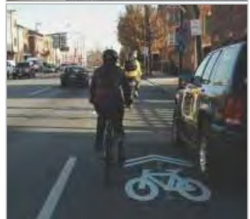
Top: Wide outside lane (14 ft.) with a sharrow, allowing enough room for cars to safely pass bicyclists. Source: MORPC. Hilliard, OH.
