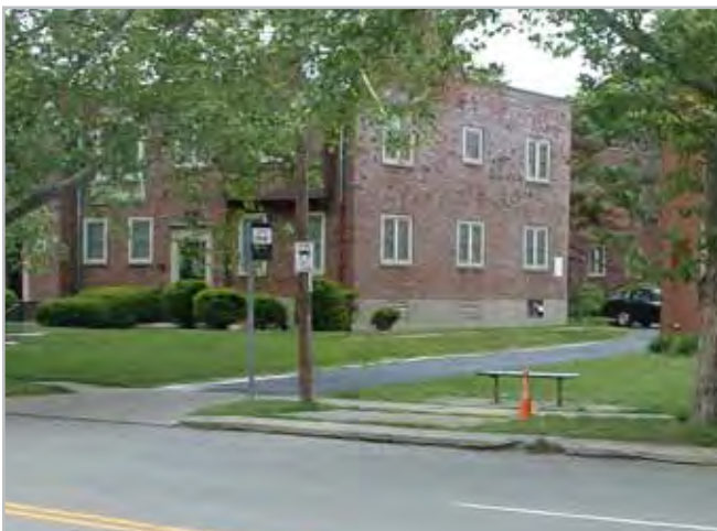
A single curb cut leads to parking in the back of the building, reducing the overall length of the curb cut. Source: MORPC. Columbus, OH.
