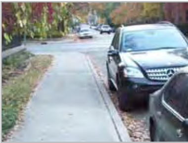
Vertical curbs discourage parking on sidewalks. Source: MORPC. Columbus, OH.
