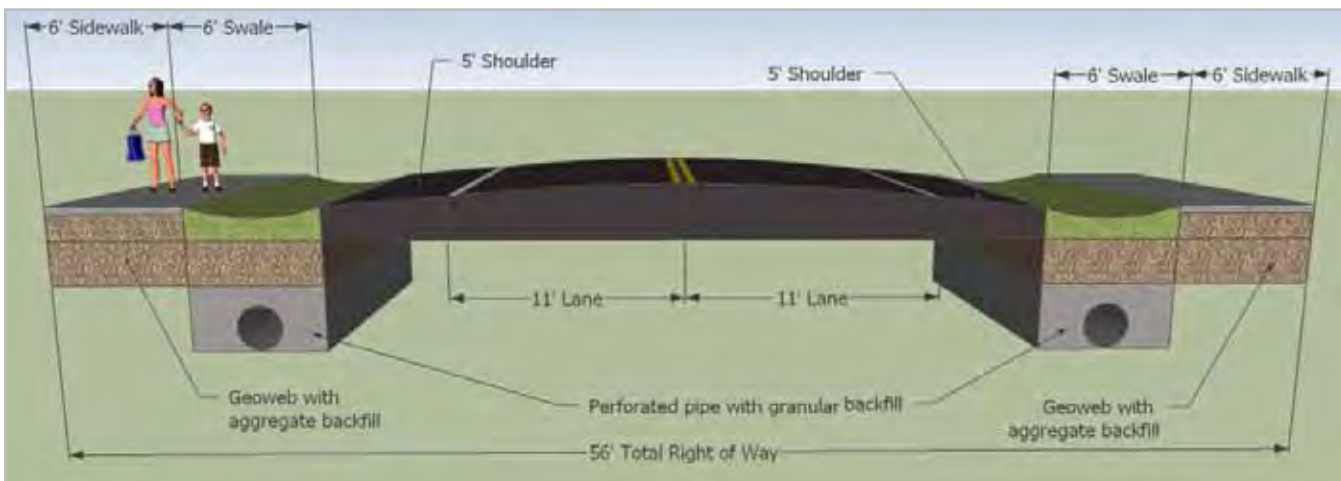
Road cross-section with 6' swale. Source: MORPC.
