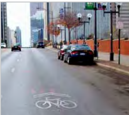
Properly positioned sharrow with on-street parking. Source: MORPC. Columbus, OH.
