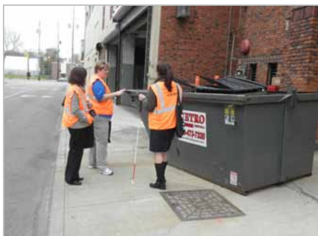
The pedestrian zone includes the corner of a dumpster, which is hazardous to blind pedestrians. Source: MORPC. Cleveland, OH.
