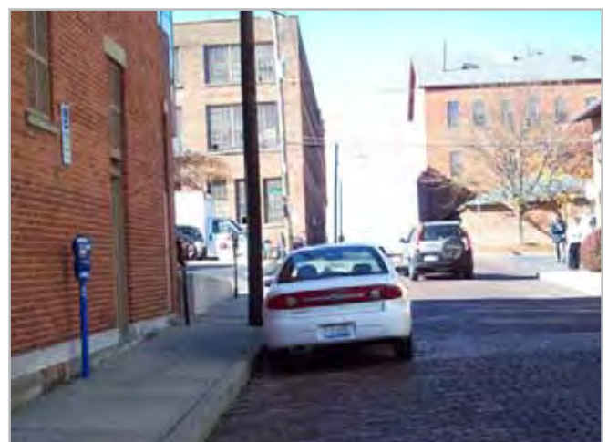
An effort has been made to keep obstacles out of the pedestrian zone, but it remains less than the recommended 5 feet. Source: MORPC. Columbus, OH.
