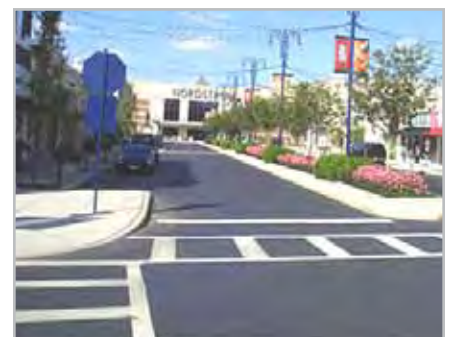
The curb extension on the left shortens the pedestrian crossing distance. Source: PBIC Image Library/Burden, Columbus, OH.
