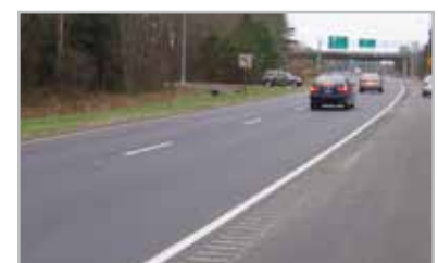
Narrow rumble strips on the left side of a wide shoulder leave sufficient space for bicyclists to use the shoulder. Source: Andrew Bossi. Salisbury, MD.
