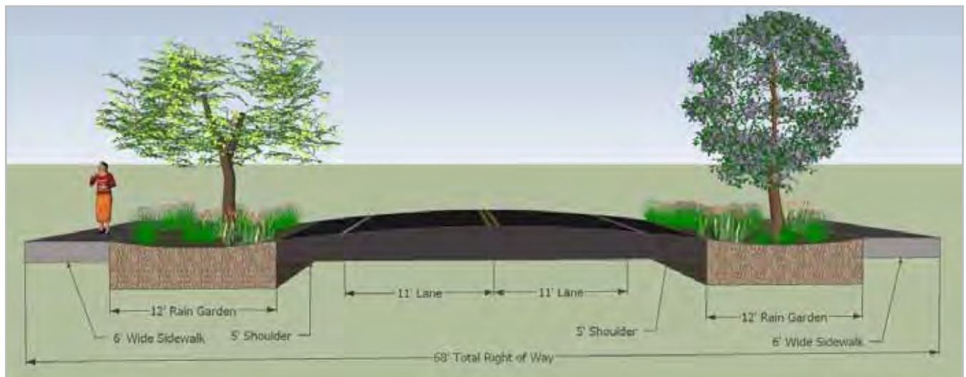
Road cross-section with a 12' rain garden. In this example, the rain garden also serves as a buffer between cars and pedestrians. Source: MORPC.
