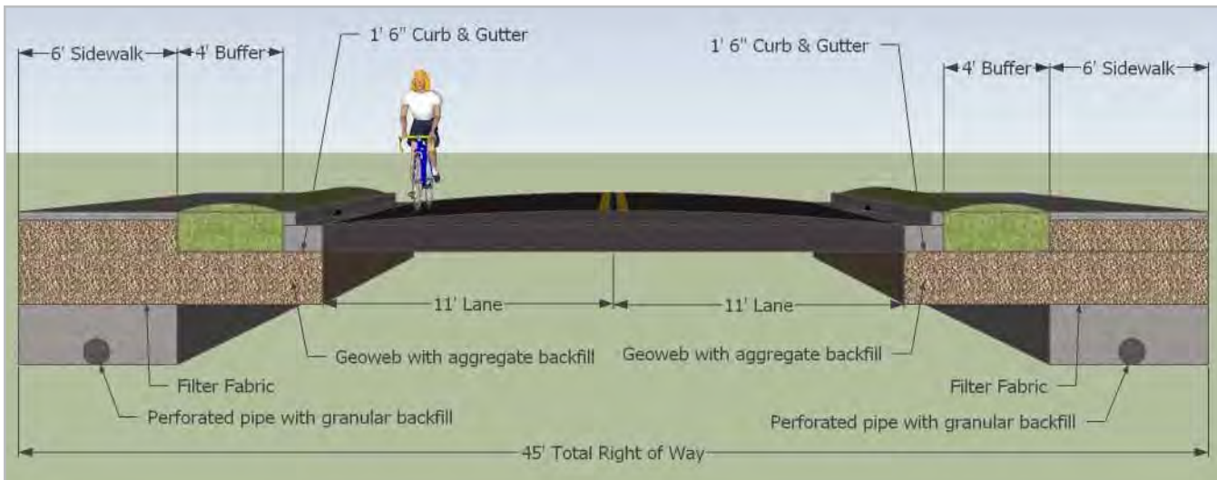
Road cross-section with 1' 6" curb and gutter. Source: MORPC.
