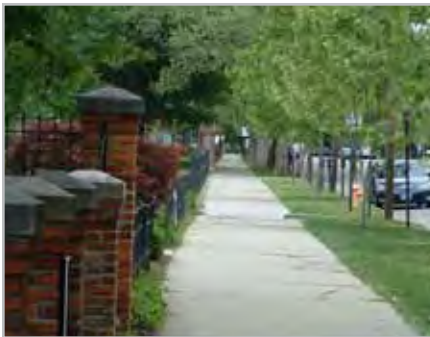
Small trees along the concrete sidewalk ensure shade for pedestrians, but will not crack the sidewalk. Source: MORPC, Columbus, OH.
