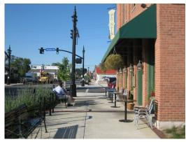
Sidewalk buffers are strips of grass or other greenery to provide distance between moving traffic and the sidewalk. Buffers can include street trees, which also add shade for the pedestrians. Sidewalks are safer and more comfortable to use when they have a buffer between them and traffic.
