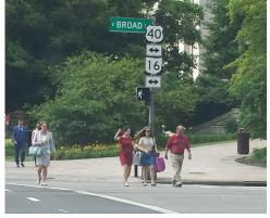
A signalized crosswalk has the same legal definition as any other crosswalk, except that it has signals to regulate the flow of vehicular and pedestrian traffic. It will have red/green traffic signals at all approaches, and may or may not have walk/don't walk signals or countdowns for pedestrians at crosswalks.
