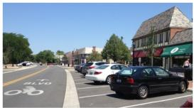
Bicycle boulevards are streets with low motorized traffic volumes and speeds which are designated and designed to give travel priority to bikes. Bicycle Boulevards use signs, pavement markings, and speed and volume management measures to discourage through trips by motor vehicles and create safe, convenient bicycle crossings of busy arterial streets. They are most effective in residential districts and near commercial corridors.
