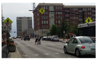
Signs may be used to indicate the presence a bicycle, pedestrian, or transit facility or to designate certain areas for those uses. Signage can include way-finding and route signage, regulatory signage, and warning signage. Some specific signage exists to provide motorized traffic with information and instruction.
