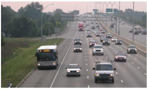
Bus on Shoulder is a program that allows authorized transit buses with trained drivers to operate on the shoulders of selected freeways at low speeds during periods of congestion in order to bypass congested traffic and maintain transit schedules. Bus on Shoulder is a low-cost treatment that can provide immediate benefits to transit whenever travel is experiencing moderate to heavy degrees of congestion.
