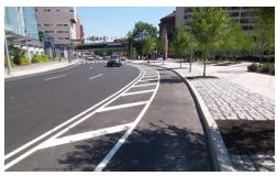
Contra-flow bicycle lanes are bicycle lanes designed to allow bicyclists to ride in the opposite direction of motor vehicle traffic. They convert a one-way traffic street into a two-way street: one direction for motor vehicles and bikes, and the other for bikes only. Contra-flow lanes are separated with yellow center lane striping.
