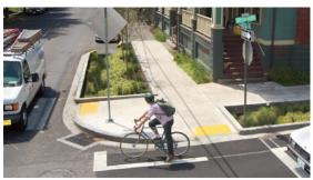
A protected intersection is an intersection with corner refuge islands, stop bars for cyclists set ahead of those for motorists, bicycle-friendly signal phasing, and bike lane setbacks that give turning motorists a clear view of crossing cyclists. The combination of these elements creates an intersection where cyclists and pedestrians are more readily seen by motorists and the non-motorized travelers have shorter distances to travel to cross the street.
