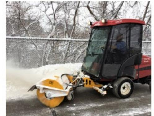
**Lawn mower tractor (converted to winter maintenance vehicle) with broom**
