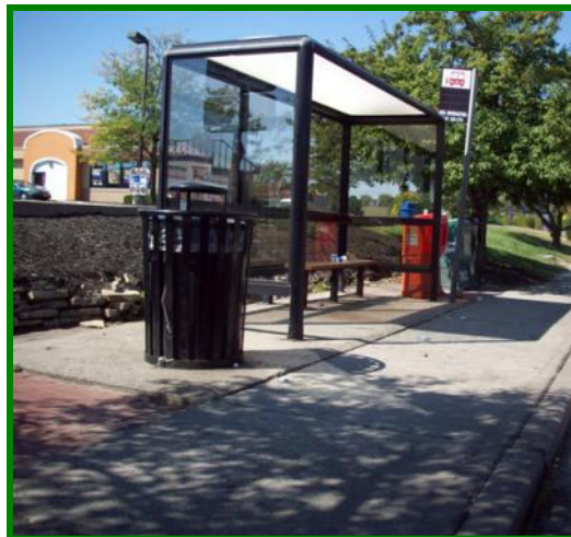
◀ This sidewalk corridor includes a curb, pedestrian, and furniture zone in Columbus, OH. (Photo: MORPC, 2010) • The furniture zone has been moved behind the pedestrian zone so that the bus shelter, garbage container, and news kiosks do not block the pedestrian zone.
