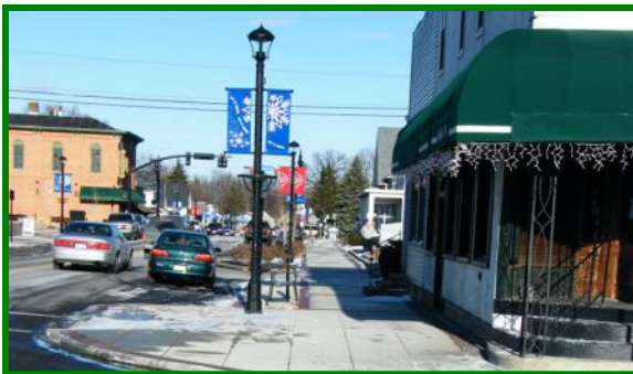
▲ The furniture zone shown here in Hilliard, OH includes benches, shrubs, and light poles. (Photo: MORPC, 2010) • The pedestrian zone is also outlined with red brick on the sidewalk.
