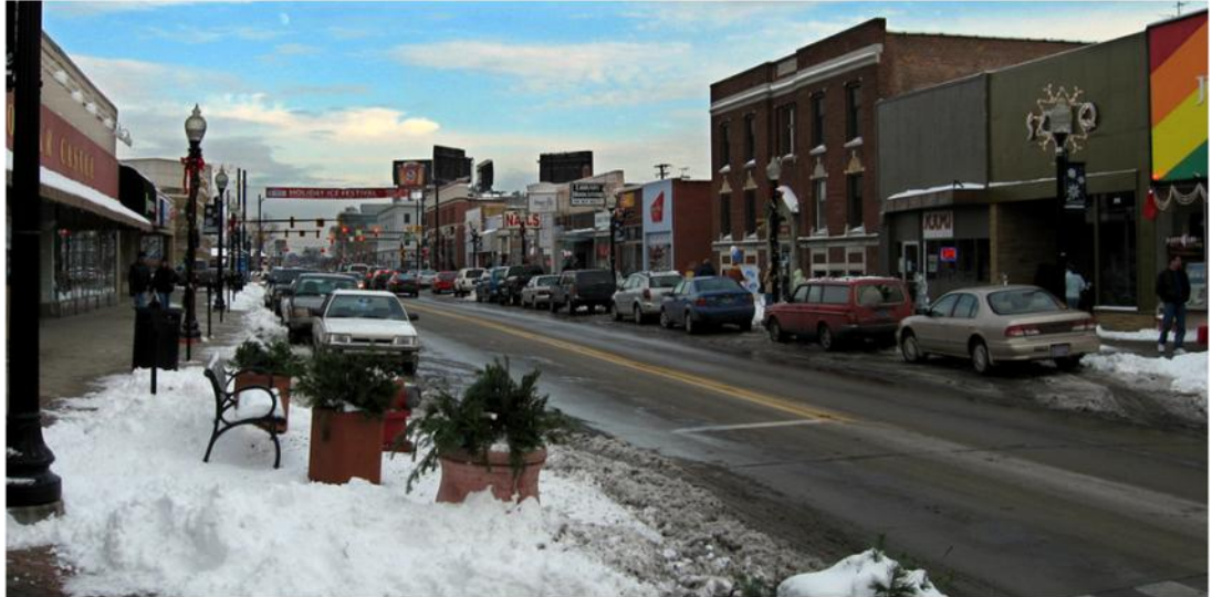
▲ Ninth Street in Downtown Ferndale after the road diet. Note that each side of the road has one parking lane and one travel lane. (Source: English Academic Wikipedia website )
